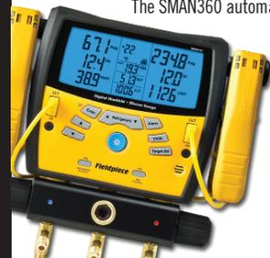
The SMAN360 automatically calculates target superheat, so HVACR professionals don't have to worry about guesswork or manual calculations. With the SMAN360 you also get a built-in micron gauge with resolution from 50 to 9,999.
